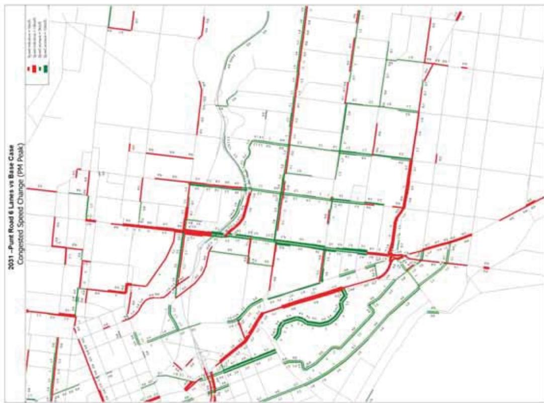
Figure 24: Change in 2031 congested travel speed - morning peak hour (6 lane vs Base Case)
